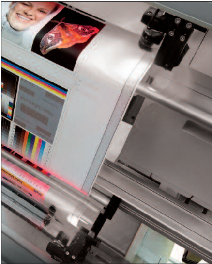
Monitored by video cameras, the DJet prints with high-precision front-to-back registration.
