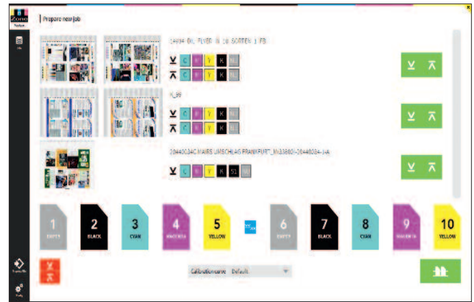
Simple assignment of printing inks to the right printing unit and selection of the appropriate calibration curve.
